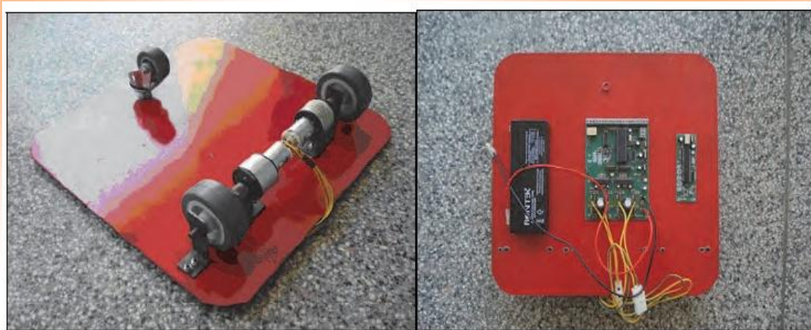
Fig. 24. The mechanical structure of the Emmy III second prototype
